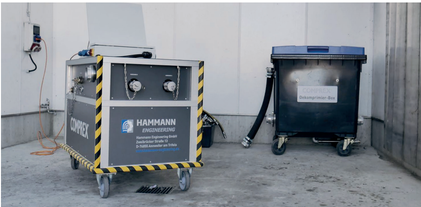
Fig. 2. A manufacturer of preforms for PET bottles used an MCU-300-series Complex unit and a corresponding decompression box © Hammann
